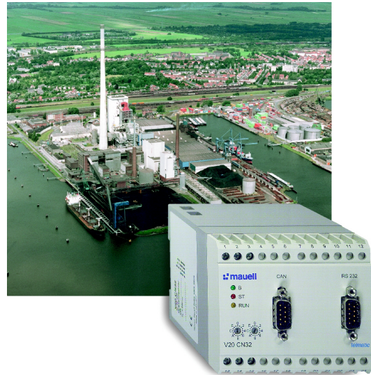
Figure 1: Coal conveyor plant of the harbor power plant, City of Bremen/Germany, controlled by a CANopen-based automation system with distributed intelligence (Foto: Helmut Mauell GmbH).
