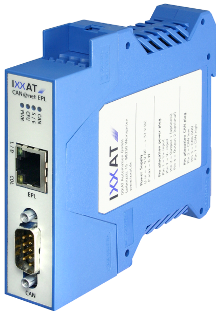
Figure 9: ETHERNET Powerlink / CANopen gateway
