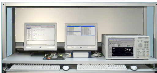
Figure 5: C&S CAN / CAN FD Automated Test System.
