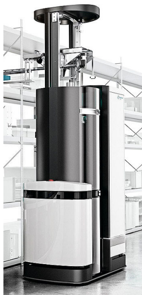
Figure 2: The Toru picker self-driving logistics robot from Magazino using CANopen motion controllers by Faulhaber is a typical example of a modern CANopen application (Source: Magazino/Faulhaber)
