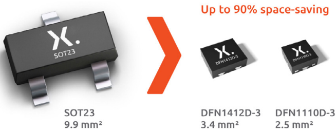
Figure 3: Leadless DFN packages reduce PCB space (Source: Nexperia)
