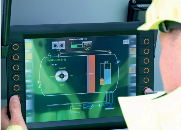
Figure 2: The robust 12-inch display CR1200 installed in the external control cabinet of the vehicle for visualisation and setting of all machine parameters (Source: ifm)
