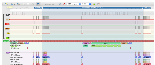
Figure 8: CAN traffic before driver optimization (Source: Ian Tabor)
