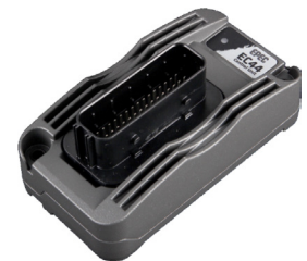
Figure 2: The EC44 has a 32-bit processor and large internal memory for application and parameters. It has 16 inputs and 16 outputs with high-side current measurement, two CAN networks, and a status LED. (Source: Epec)
