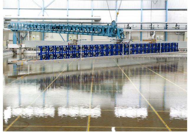
Figure 3: CAN-connected fans are used to create wind for tests (Source: Marin)
