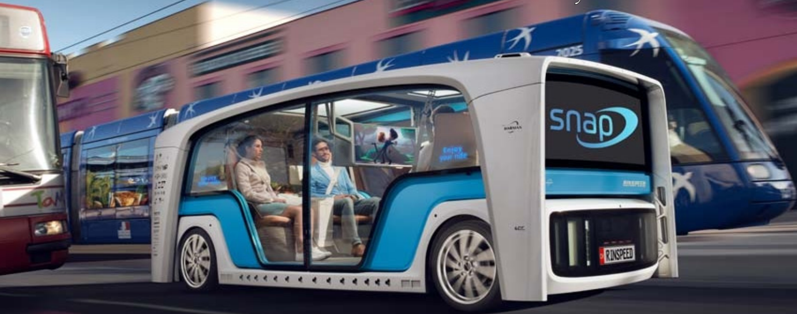
Figure 1: The Snap concept car comprises a chassis, the “skateboard”, and the passenger cell, the “pod” (Photo: Rinspeed)
