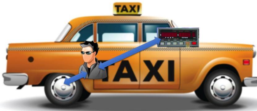
Figure 3: Man-in-the-middle attack between wheel and meter (Source: Esacademy)
