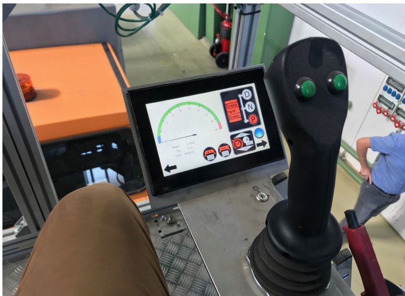
Figure 2: The control of the stilt tractor is realized with an operating and control unit of type D1520, to which an analog joystick is connected (Source: Graf-Syteco)
