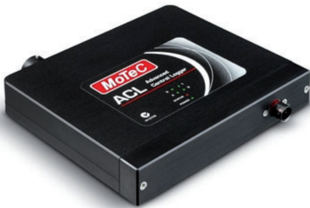
Figure 4: The ACL logger communicates via CAN with multiple SVIM input modules (Source: Motec)
