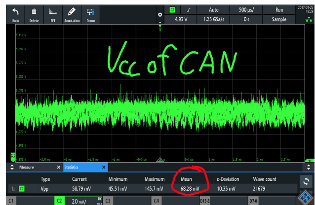
Figure 2: More accurate measurement results applying the right vertical settings and advanced frontend technology (Photo: R&S)
