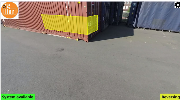
Figure 4: Critical objects are marked in the camera image (Photo: ifm)
