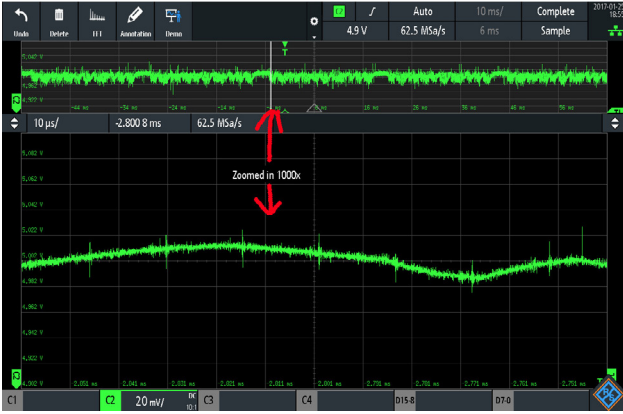
Figure 3: Low- and high-speed coupled events are captured using long memory (Photo: R&S)
