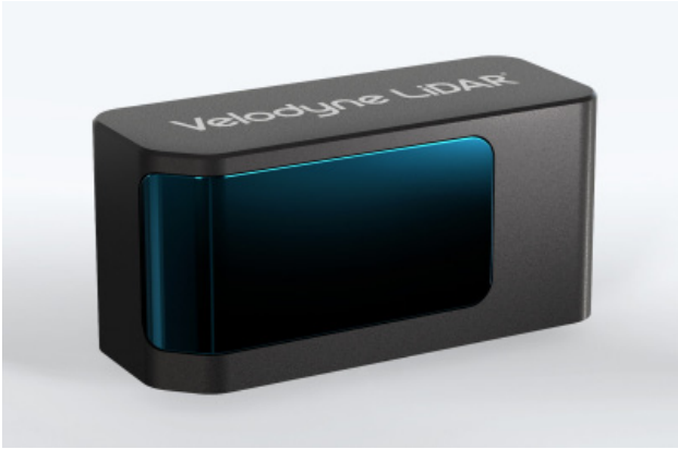
Figure 1: The Velarray lidar uses Velodyne's proprietary ASICs and comes in a package size of 25 mm x 50 mm x 55 mm; it provides a 120-degree horizontal and 35-degree vertical field-of-view with a 200-m range (Photo: Velodyne)
