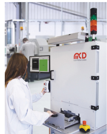
Figure 2: Placing a module in the test cell tray (Photo: MCD)
