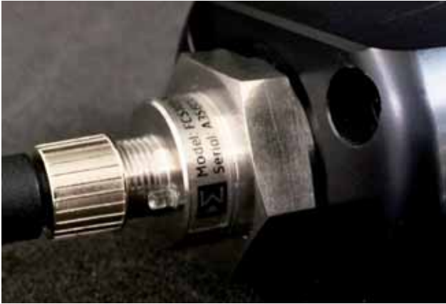
Figure 5: The sensor vanishes almost completely after installation into an appropriate cavity
