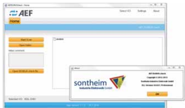
Figure 2: The Isobus Check Tool collects important diagnosis information of different ECUs on the bus
