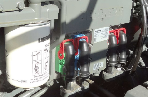
Figure 5: Diesel engine ECU with in-built cable clamps. Source: TE Connectivity
