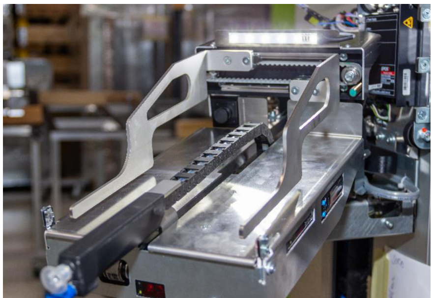
Figure 4: The gripper system is equipped with a E065 chain; The chain also carries a vacuum line for suctioning the packaging to be picked (Source: Igus)
