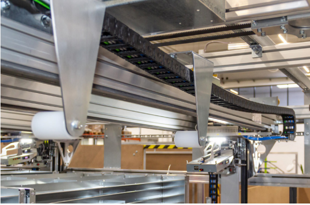
Figure 3: Energy and CAN signals reach the RBG axes through energy chains (Source: Gollmann Kommissioniersysteme)
