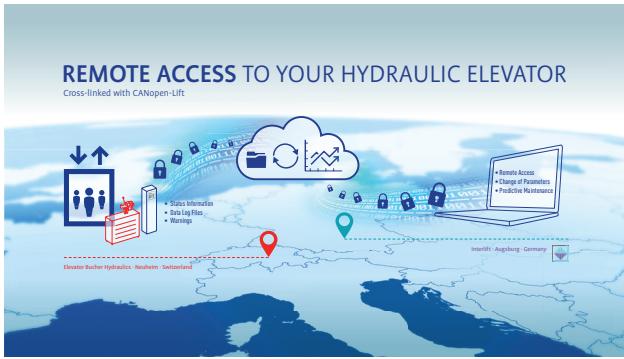
Figure 3: The valve technology helps users to implement predictive maintenance concepts thanks to a continuous awareness of the condition of the equipment (Source: Bucher Hydraulics)
