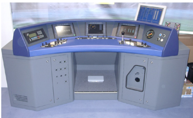
Figure 2: Demonstration driver desk exhibited on the Innotrans 2004 (Source: Deuta)
